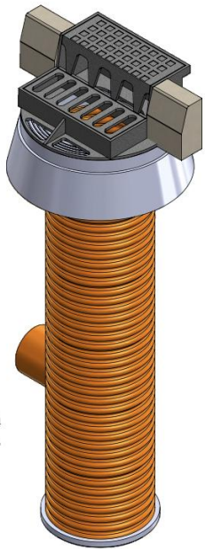
Plastic well DN/ID 400 acting as a sewage drain with settling tank. Surface finish made from T3/425 relief cone and TX/4052/AP adapter placed under full-iron kerb and roadway drain. T4/400/P covering constitutes as a bottom.
